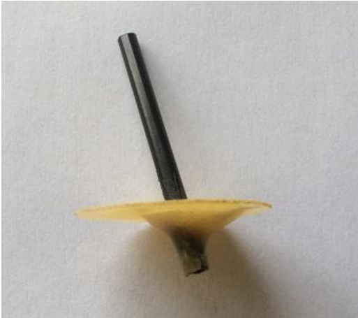
Above is an example of a breather tube fitted in the rear patch of GBR 42 at the Garda World Championship 2016
