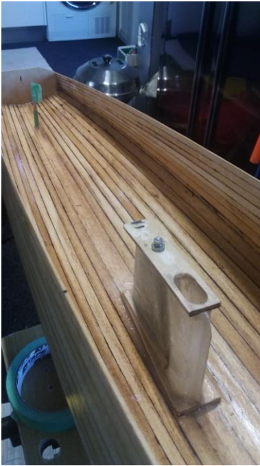
Internal fittings start. Keel and mast tube made from fibreglass and rudder tube in SS. Bracing added in 3/32 ply
