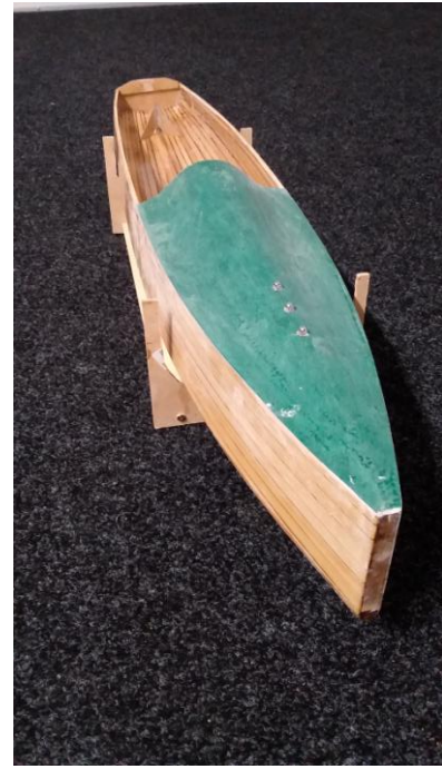
Cockpit sides being glasses after being formed. Foredeck glued to canoe sanded and prep'd
