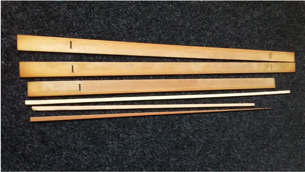
Raw material source for the hull is old timber venetian blinds. Teak slats are 3.5 to 4 mm in thickness due to fading and timber decomposition. Each plank cut to nominal 10mm width with craft knife through each plank shaped to fit
