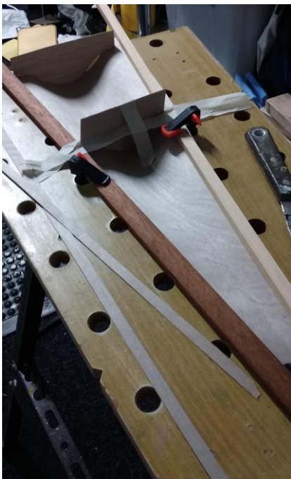
Fore deck being bent to curved frame with stiffeners added and reinforcing for rigging screws. Photo 2 shows Mast ram being glued. Outside skin with timber stain and protective epoxy to highlight grain.
