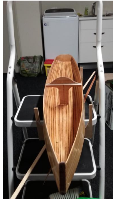
Internal fittings start. Keel and mast tube made from fibreglass and rudder tube in SS. Bracing added in 3/32 ply
