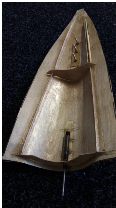
Fore deck being bent to curved frame with stiffeners added and reinforcing for rigging screws. Photo 2 shows Mast ram being glued. Outside skin with timber stain and protective epoxy to highlight grain.
