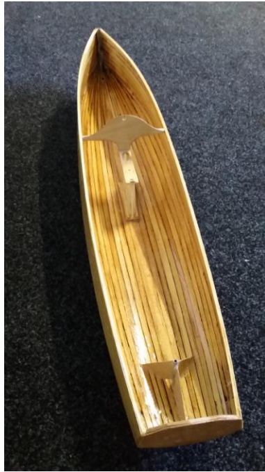
Internal fittings start. Keel and mast tube made from fibreglass and rudder tube in SS. Bracing added in 3/32 ply
