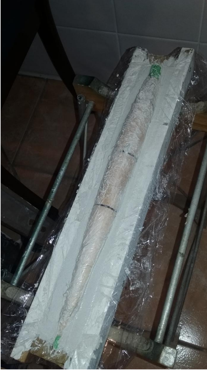
A turned balsa keel bulb was wrapped in glad wrap then inserted into a mould containing paving sand and cement. Once set the bulb was poured with lead in two parts
