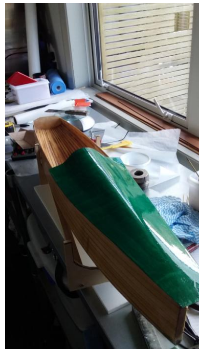
Fore deck being bent to curved frame with stiffeners added and reinforcing for rigging screws. Photo 2 shows Mast ram being glued. Outside skin with timber stain and protective epoxy to highlight grain.
