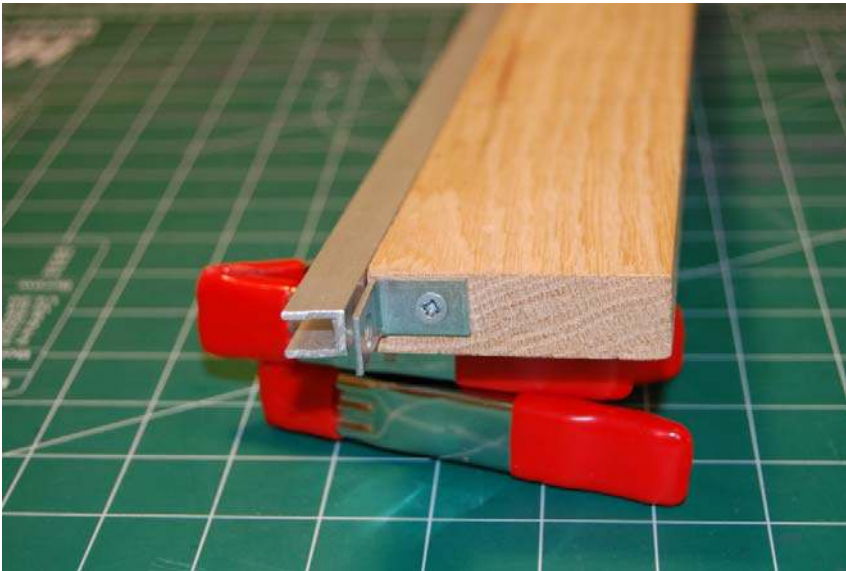
The “L” brackets are mounted at the ends and allow the spring clamps to hold the bar flat to the wood base.
